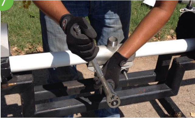
If necessary to reposition, loosen nuts prior to moving saddle and then retorque.
