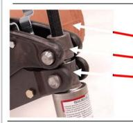
Turn adjusting screw until outer collar is at it's lowest limit of travel. Do this for EACH cut.
