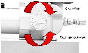
9. Turn valve clockwise on the pump until it is HAND TIGHT. DO NOT USE A WRENCH. Make strokes necessary to snap pipe. Turn knob counterclockwise to release valve after cut to retract piston.
