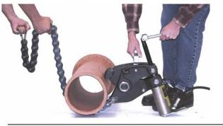
2. Slide chain under pipe at location of cut.
