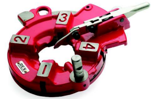
MODEL NO. 60118 DIE HEAD, AUTOMATIC OPENING, 1/2"-2" NPT
