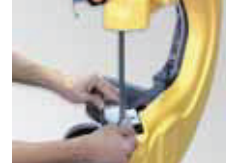
Contour cutting for small steel materials.
