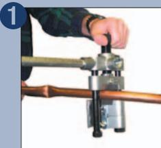
1 To shut off flow, place tool over tube, swing dies onto guide rods and latch. Tool handle can be repositioned for confined working spaces.
