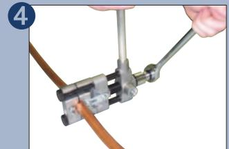
4 Use ratchet to compress reforming dies. Die shape will prevent over-forming and fatiguing tube walls as flow is restored.
