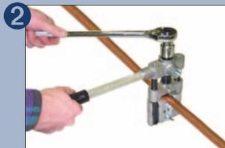
2 Use ratchet to compress Shut-Off dies. Needs only enough compression to stop flow. Watertight closure is maintained while the tool (or holding clamp) is affixed to the tube.
