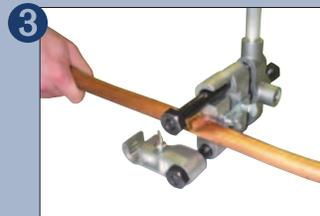
3 To restore flow, remove tool and rotate 90°. Using the bottom two dies, reattach tool so that the reforming dies are properly located around flattened tube edges.
