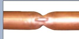
Our unique reforming dies prevent flattened tube edges from overworking and cracking. The loss of head is no more than through a 90° elbow.
